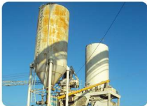
Elba : Fix/Wet Capacity: 60m3/hour
